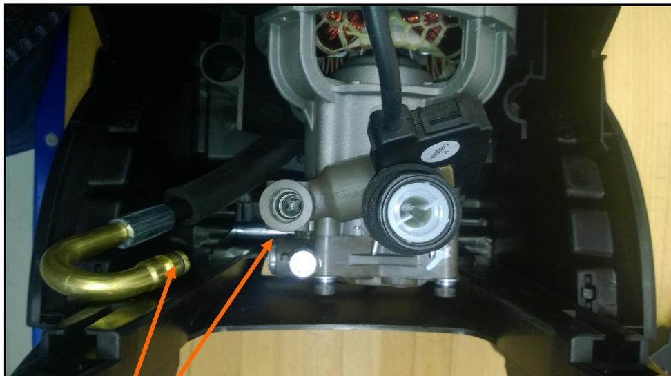
**Disassembly / assembly of the hose reel / internal hose - X-TRA models.**
