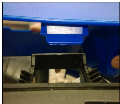
**Disassembly / assembly of pump cover.**
